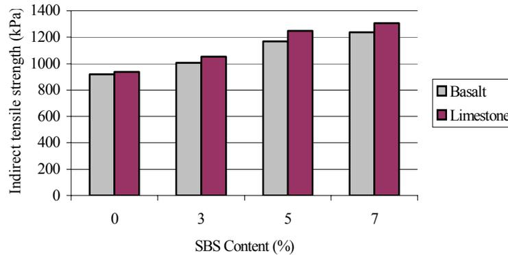
**Figure 2.** Indirect tensile strength of the mixtures
