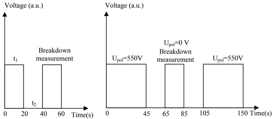
**Figure 2.** (a) The voltage pulses when polarization potential was not applied. (b) The voltage pulses when polarization potential was applied.  $t_1$  indicates duration time of discharge,  $t_2$  indicates time between two measurements
