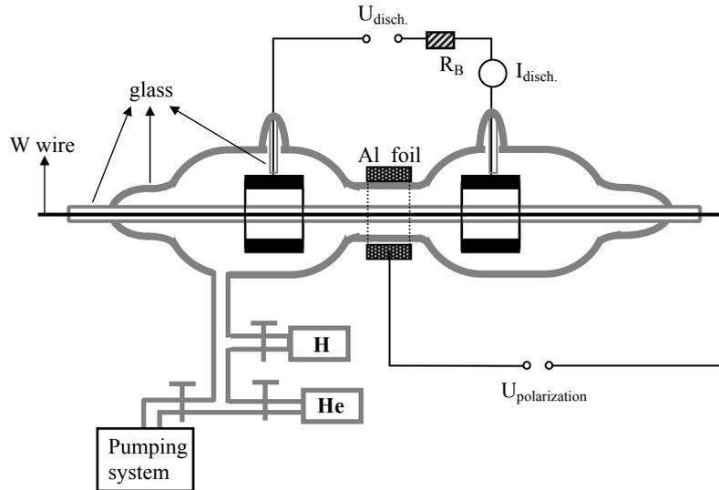
**Figure 1.** Schematically experimental device. H and He gas tubes besides various gas tubes can be mounted to the system
