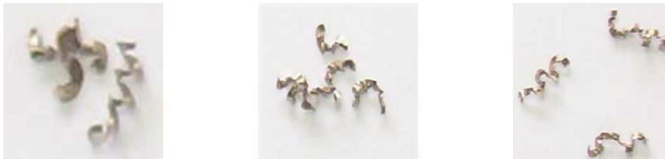
Figure 5. Typical chip forms (a; 100m/min, b; 150 m/min, c; 200 m/min cutting speed, feed rate 0.2 mm/rev and 2 mm depth of cut)
