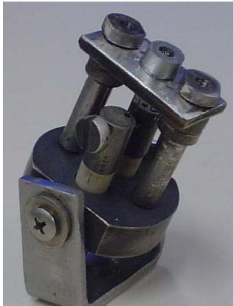
**Figure 1.** Photo of the cathode showing the filament placed inside the Wehnelt
