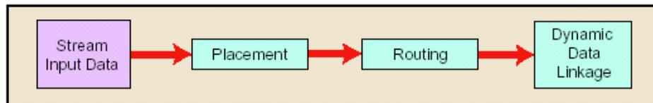
**Figure 4.** Process involved in one-line diagram generation
