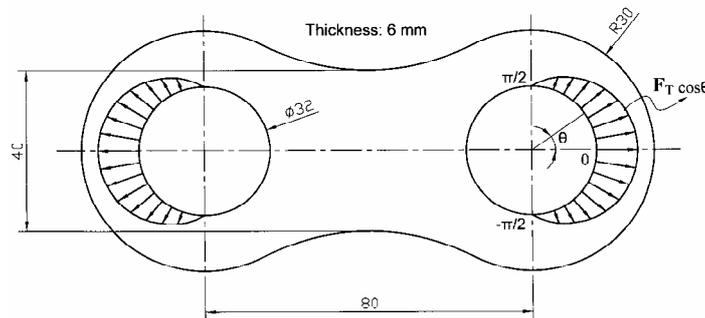
Figure 1. The chain link with fully dimensioned
