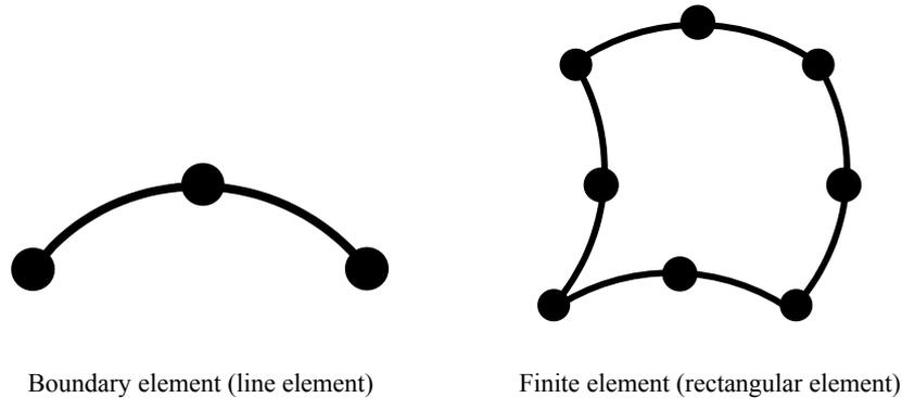
Figure 3. Quadratic elements used in BEM and FEM
