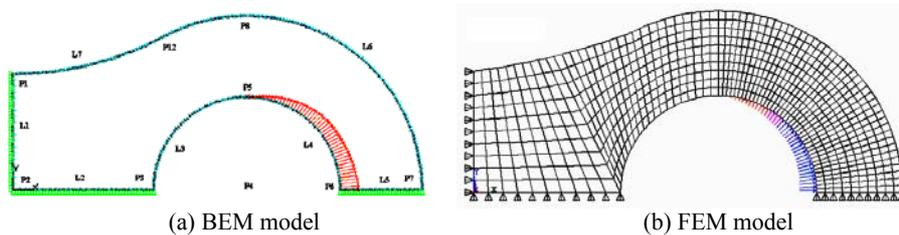
Figure 2. Chain link model in numerical methods
