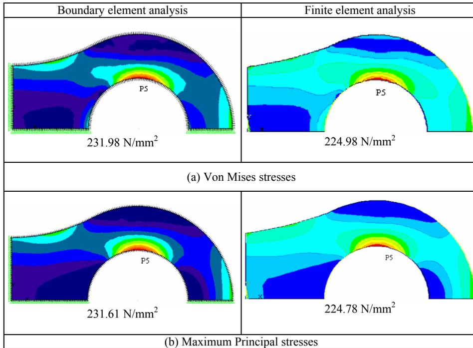
**Figure 4.** Stress distributions on the chain link
