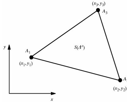
**Figure 2.** A triangular element with three vertex coordinates
