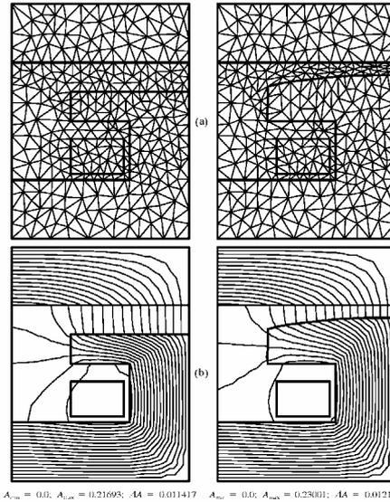
**Figure 19.** Computational results for the parametrization with 6 variables (in Figure 1.15) applied to the heavily-saturated, salient-pole generator to obtain a sinusoidal flux-density distribution with the magnitude of 1.0 T: (a) deflected mesh geometry; (b) flux lines for the initial and the optimized pole shapes
