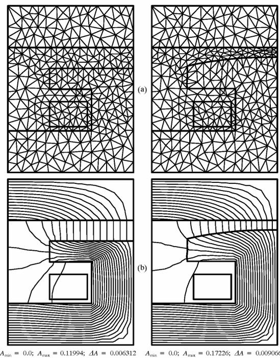
**Figure 16.** Computational results for the parametrization with 6 variables (in Figure 12) applied to the moderately-saturated, salient-pole generator to obtain a sinusoidal flux-density distribution with the magnitude of 0.75 T: (a) deflected mesh geometry; (b) flux lines for the initial and the optimized pole shapes
