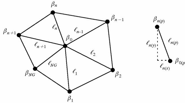
**Figure 5.** Iterative scheme to calculate displacement weights of free-moving nodes from those of their neighbors
