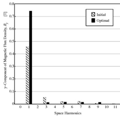
**Figure 18.** FFT analysis showing the space-harmonics of the air-gap magnetic flux density distribution in Figure 17
