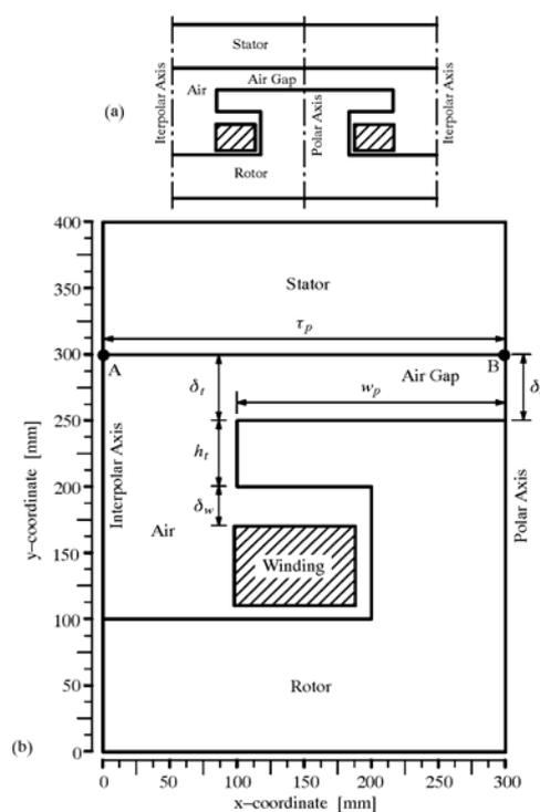
**Figure 10.** Magnetic-circuit model of a salient-pole synchronous generator: (a) the full pole-pitch geometry including the stator, rotor, air, pole and field-winding regions; (b) the solution domain and geometric dimensions of one-half of the pole pitch
