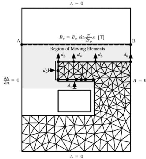
**Figure 12.** Definition of the field and optimization parameters applied to the mesh model in Figure 11. Dirichlet and Neumann boundary conditions, and the user defined rectangular region (the light-grey region) of moving mesh including 158 nodes
