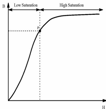
Figure 7. A Typical B-H characteristic curve of a nonlinear magnetic material with low- and high-saturation regions
