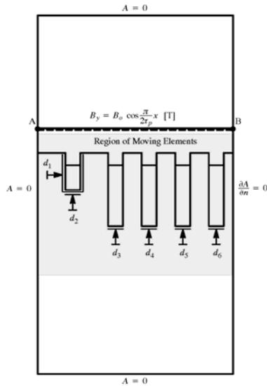
**Figure 25.** Definition of the field and optimization parameters used for the mesh shown in Figure 23. Dirichlet and Neumann boundary conditions and the user defined rectangular region of moving mesh including 424 nodes
