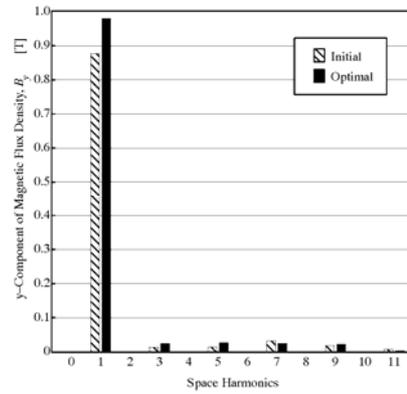
**Figure 21.** FFT analysis showing the space-harmonics of the air-gap magnetic flux density distribution in Figure 20
