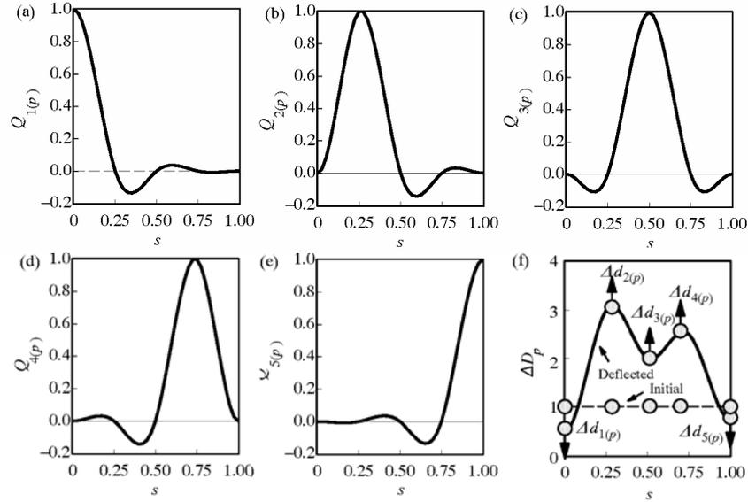
**Figure 4.** Modeling a five-knot device contour using basis functions: (a)-(e) the cubic-spline basis functions of each knot; (f) the initial contour (dashed line) is deflected after applying incremental displacements to each knot
