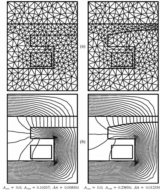
**Figure 13.** Computational results for the parametrization with 6 variables (in Figure 12) applied to the unsaturated, salient-pole generator to obtain a sinusoidal flux-density distribution with the magnitude of 1.0 T: (a) deflected mesh geometry; (b) flux lines for the initial and the optimized pole shapes
