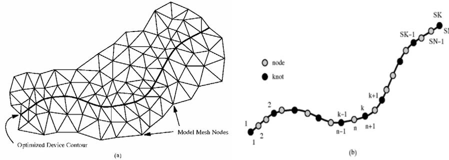
**Figure 3.** Modeling the optimized contour: a) triangular mesh and device contour; b) numbering nodes on the device contour and the user defined knots
