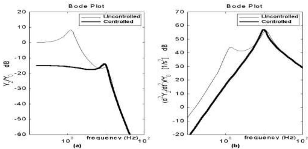
Figure 5. Frequency response of the body displacement and acceleration
