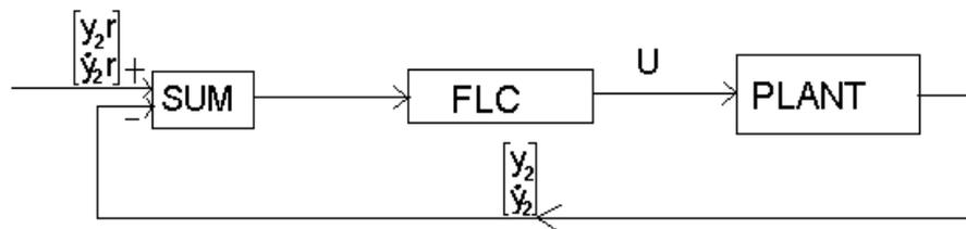
Figure 3. Closed loop model of the vehicle with fuzzy logic controller
