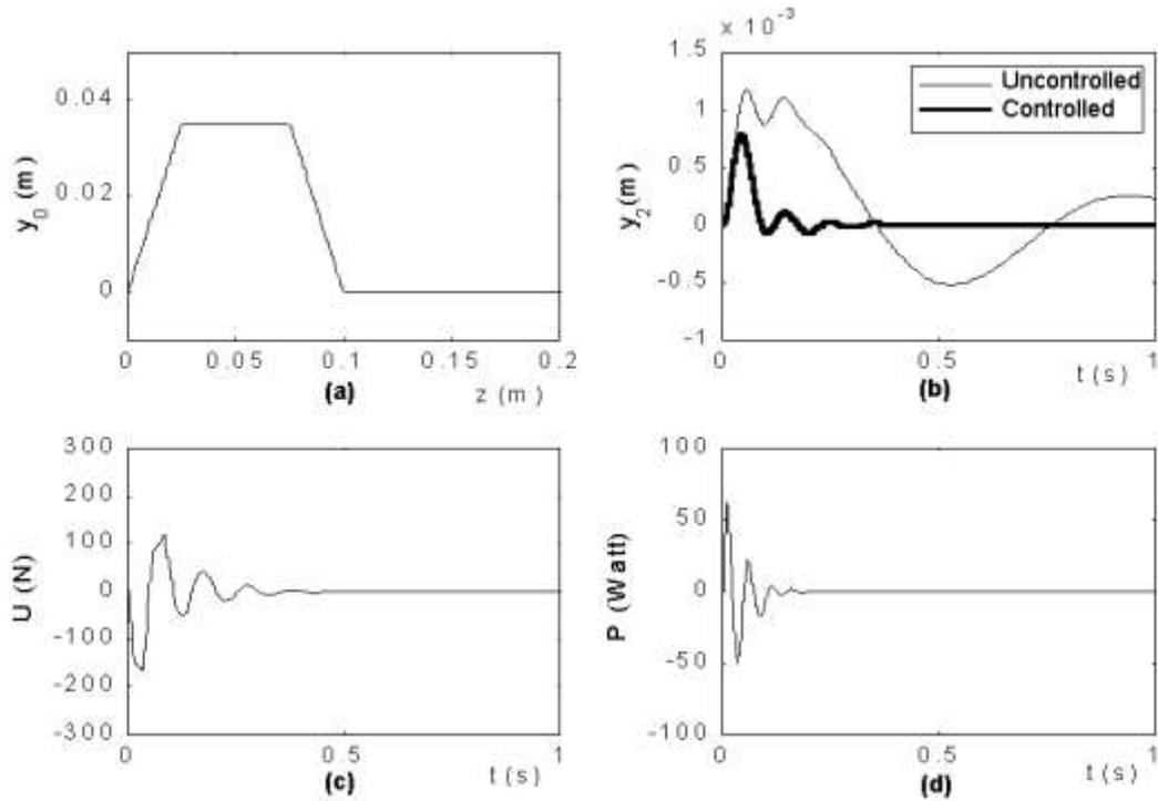
Figure 4. The system response of the vehicle in case of bump road surface input
