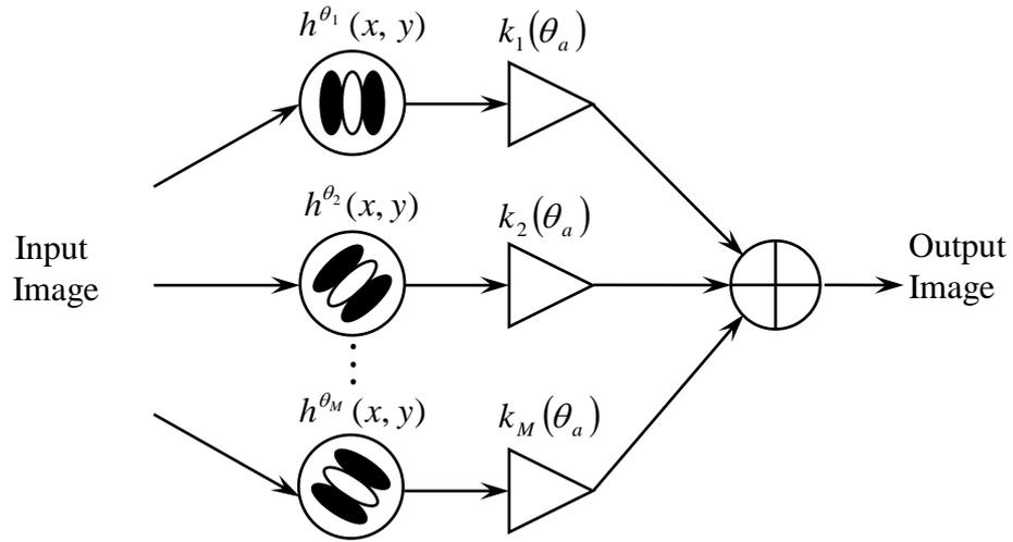
Figure 1. Steerable filter system block diagram.
