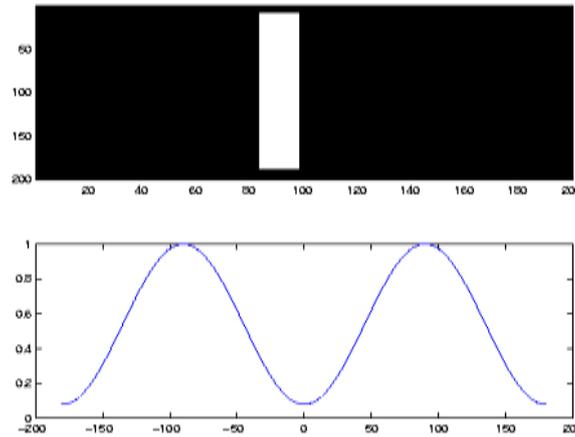
**Figure 2. (a)** Test image, **(b)** oriented energy with respect to angle for a pixel on the vertical line.
