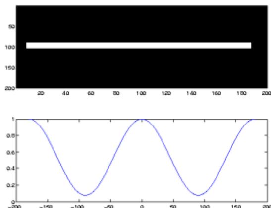
**Figure 3. (a)** Test image, **(b)** oriented energy with respect to angle for a pixel on the horizontal line.
