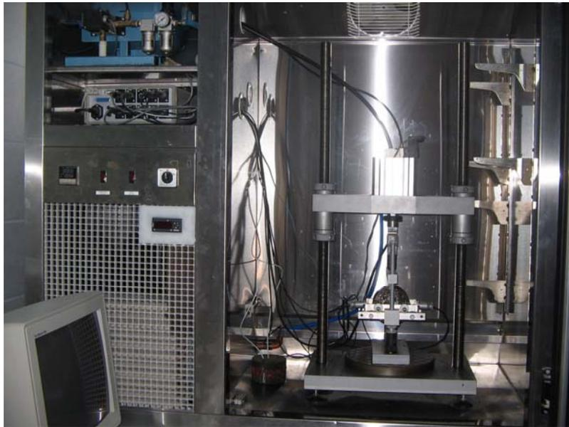
**Figure 3.** Universal testing machine
