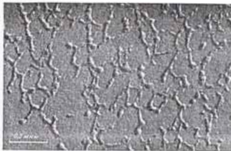
Figure 30. Electron micrographs of PVEP-BGG polycomplex when n_{BGG}/n_{PE}=2 , DP=0,95.10 3 . (Sample preparation as in the case of BSA-PVEP).
