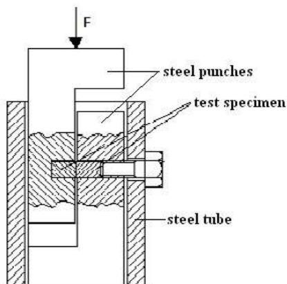
Figure 3. Schematic illustration of the shear test apparatus
