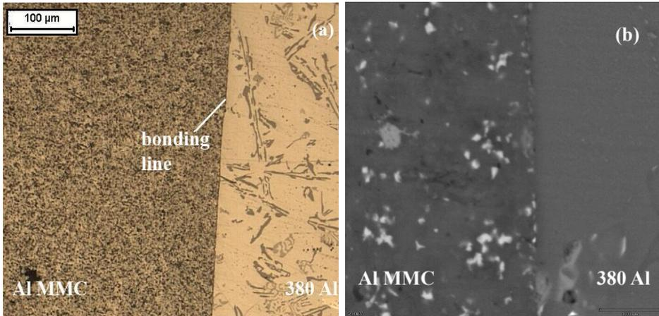
**Figure 7.** Optical micrographs of the bonding interface of the samples diffusion bonded at 560°C with 3 MPa for 90 minutes (a) optical micrograph (b) SEM micrograph
